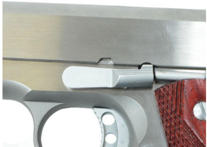
4. Push inward on the end of the slide stop shaft on the right side of the pistol and remove the slide stop from the left side.
