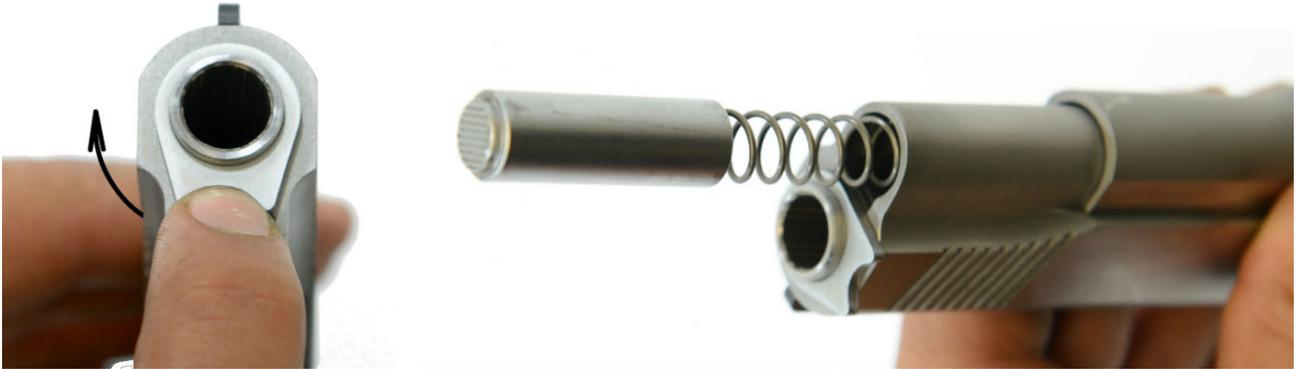
2. Carefully remove the recoil spring and cap.
