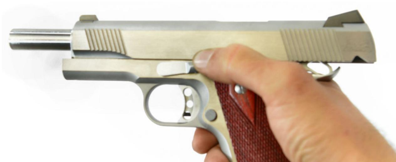
You must verify the barrel chamber and bore are free of any live rounds or obstructions. You must follow this procedure every time your firearm is inspected, cleaned, handed to another person, transported or stored. Unload the magazine by holding it with the bullet end of the cartridge pointing away from you and pressing each cartridge forward and out of the magazine. Secure all live rounds.
