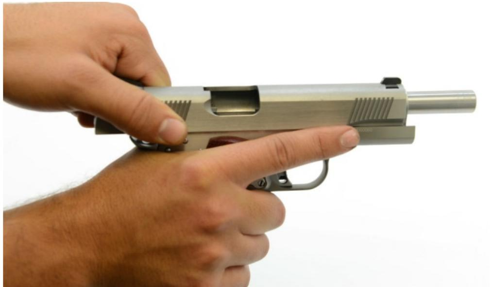
Lock the slide in the open position by allowing the slide to move slightly forward from the rearmost position while pressing the slide stop upward so that it engages the most forward of notches on the left hand of the slide; the slide stop notch.
