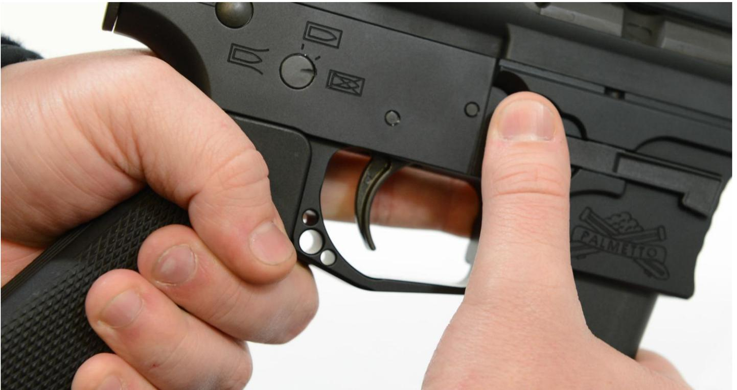
Unlock and pull the charging handle all the way out and press in on the lower portion of the bolt catch. Release charging handle. This locks the bolt in the open position.
