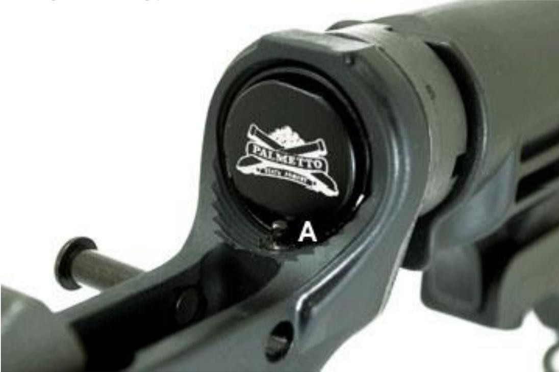
Once the spring is no longer compressed, remove from buffer tube.
