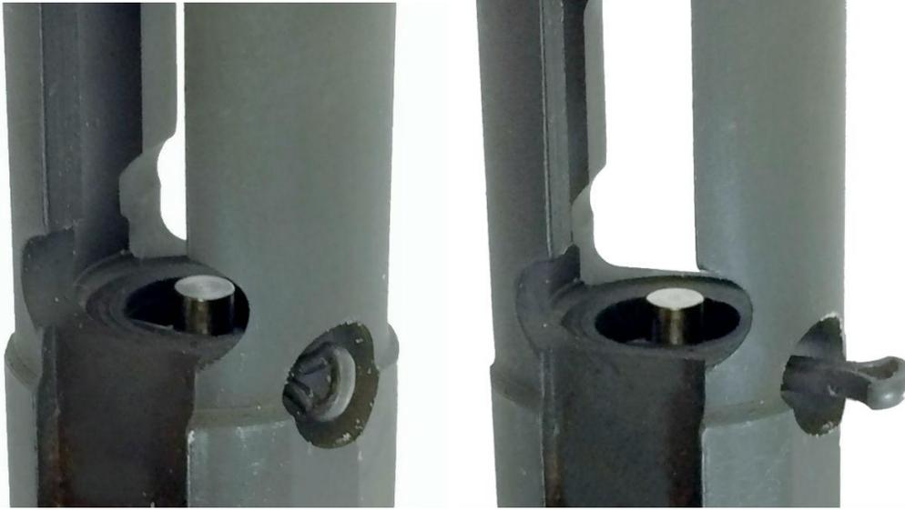
The Firing pin may now be removed from the bolt assembly. No further disassembly is required for maintenance.
