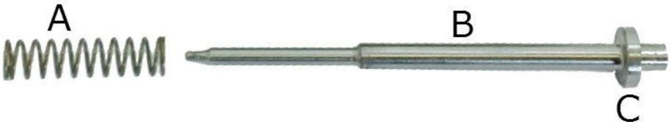
Insert Firing pin spring and Firing pin assembly into the Bolt. While pushing down on the rear of the firing pin, slide the retaining pin into the bolt behind the machined lip (C) of the firing pin, keeping the firing pin under tension and in place. Be sure the firing pin retaining pin is seated in the bolt so that the head is flush with the outside of the bolt.
