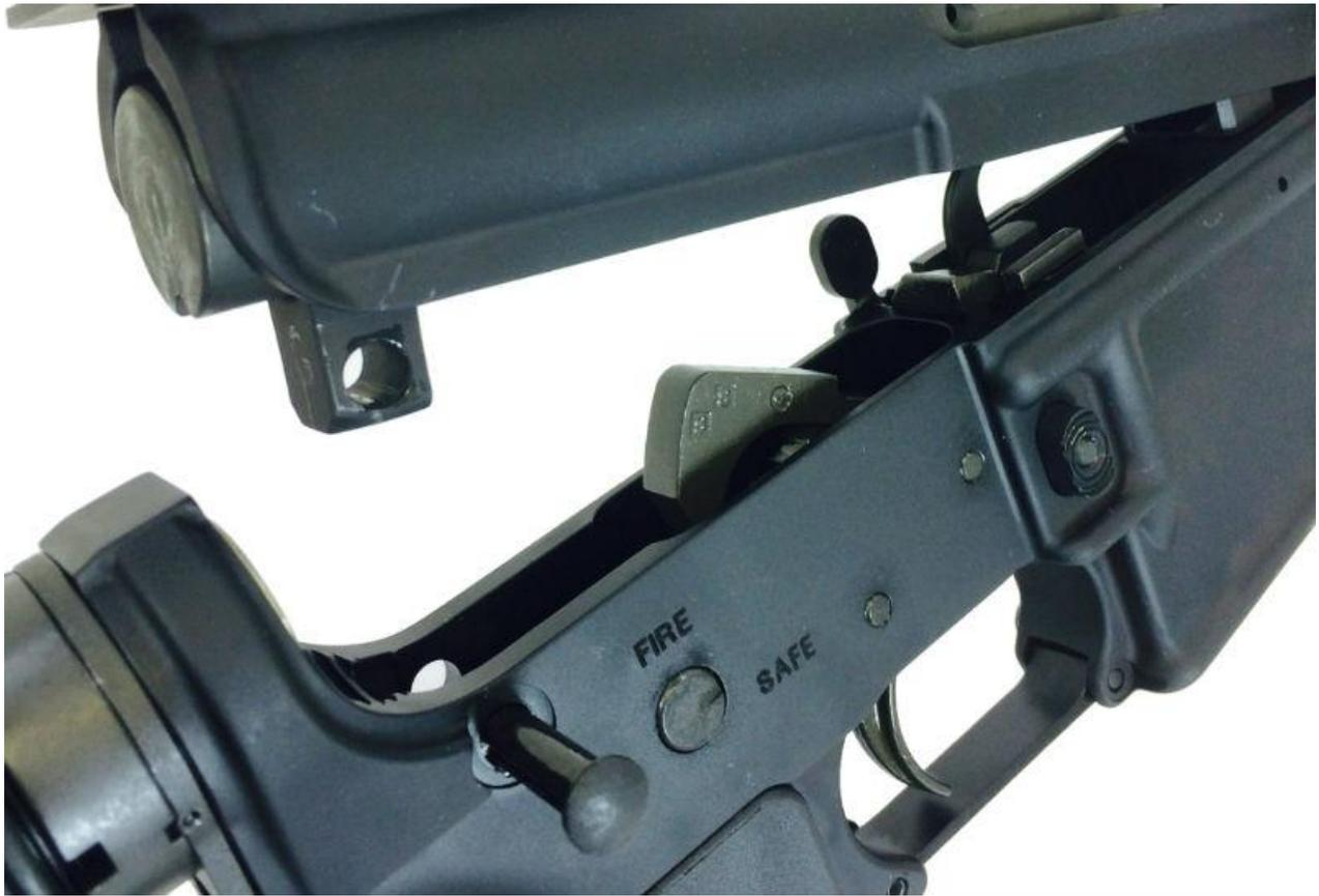
Unlatch the charging handle and pull it back, this will extract the bolt carrier group.
