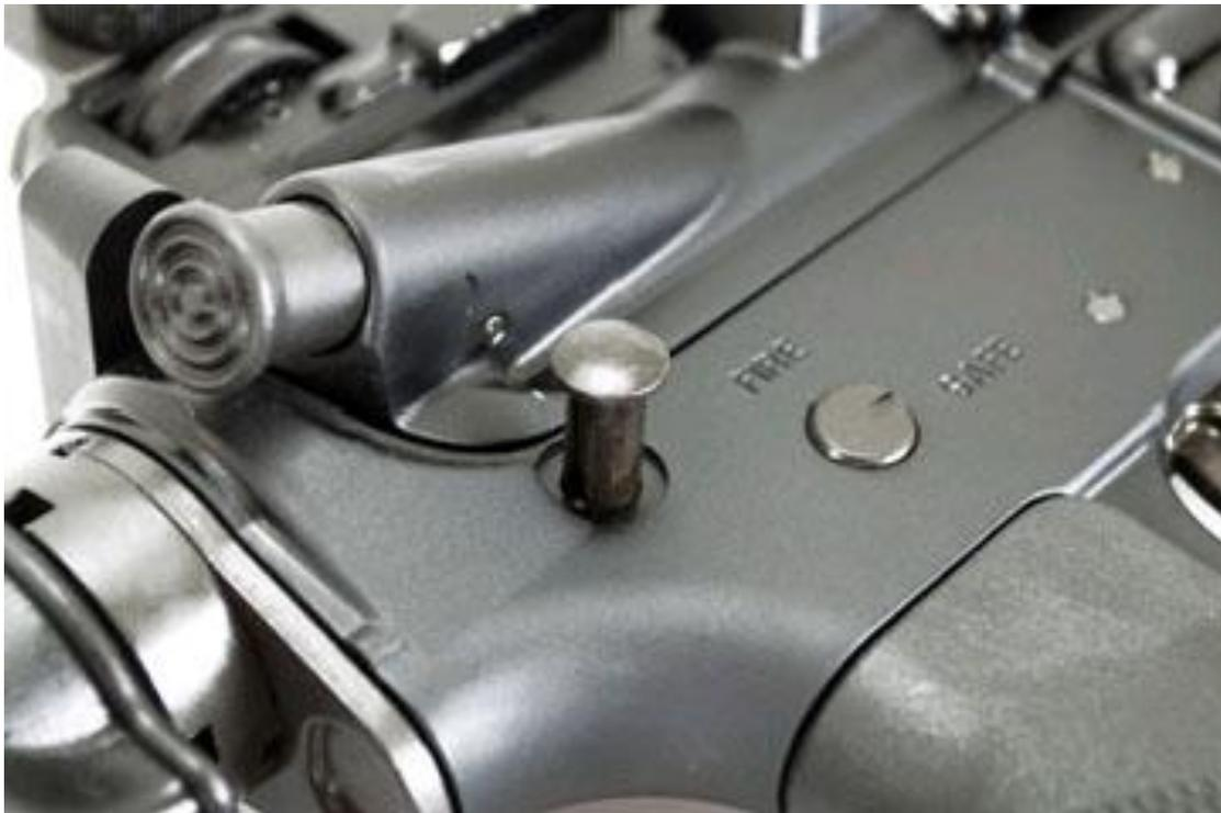
Grasp the rear of the upper receiver and pull up, allowing it to pivot on the front pin. This will expose the fire control group.
