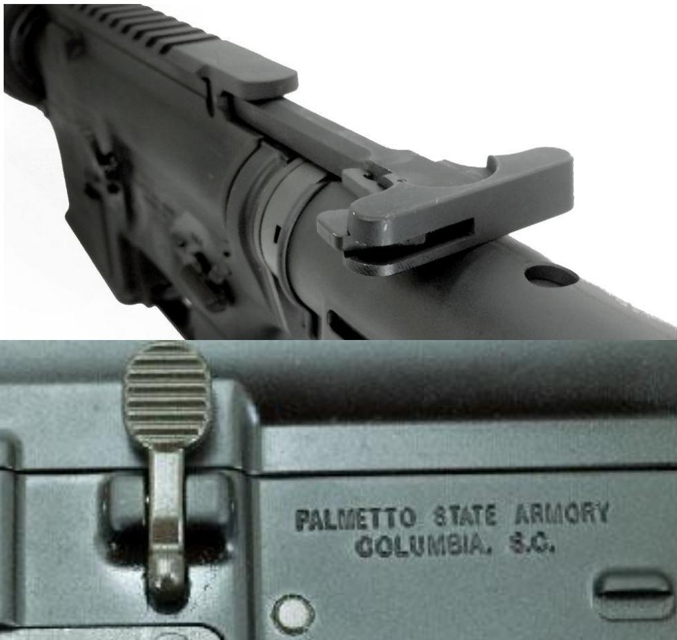
Look into the receiver through the ejection port and verify that there are no cartridges in the chamber.
